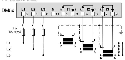
• With current and 3 single-pole isolated voltage transformers
