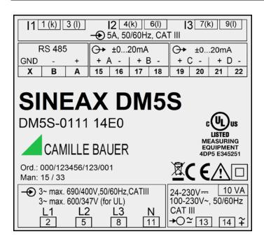
Nameplate of a SINEAX DM5S equipped with RS485 interface and 4 analog outputs
