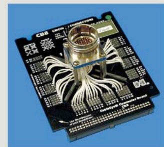
CB8 Board (Item 738) with Connector Mounted
