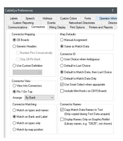
*Generic Headers* displays the result as they are found directly in the CableEye 64-pin headers. This is normally represented as B1:15, for test point 15 in bank 1. Generic headers displays everything connected to the headers and it's a perfect tool for debugging troubleshooting maps.
