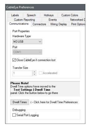
The Serial Port Logging check box in the Debugging section tells CableEye to create a log file in your ...CableEye\Software directory named CiSerialPort.log that details the communications transactions between CableEye and the test fixture. You should leave this box unchecked unless instructed to check it by CAMI support staff.
