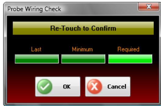
When the probe is removed from the lead and CableEye is ready to sense the confirming re-probe, a “tick” sound is played and the top field is changed to a green background.
