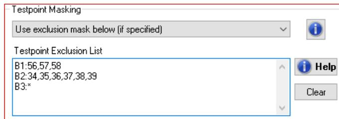
If for example, we have a connection in our cable between TPs 35 and 36 on bank 2, CableEye will not report that connection.
