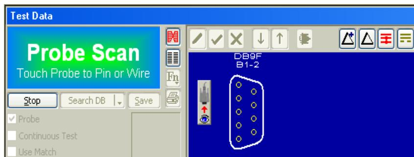
4. **Touch Pin 1 with the Probe.** A wire leading to this pin appears in the display along with a large white balloon on the right with an easy-to-see depiction of the pin number. You will also hear "Pin One" spoken if you have a synthetic voice font active in your computer.
