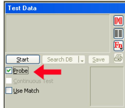
**Mode 2, Matching:** Clicking on the **Use Match** checkbox as well activates a *comparison function* enabling software to check each wire probed against the wiring loaded in the Match Data buffer. As the software detects individual flying leads you touch, it marks corresponding wiring in the Match Data as present, and stops automatically once all wiring has been seen. This “test” function will also check wire resistance if resistance values appear in the Match Data.
