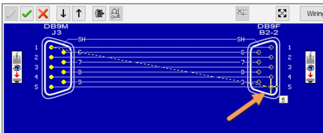
4. Once the new connection is created, **click** on the green **checkmark** and **Save** button to save the changes, just like in the netlist view.
