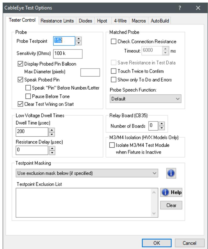
**Testpoint Masking** - You can define an exclusion list of test points, which will mask out or ignore the test points in it during testing. In other words, any connection going to these points will not be reported by CableEye. Sometimes this is useful when a specific connection is unrelated to the cable that you are testing, and you don't want it to be displayed on the report.
