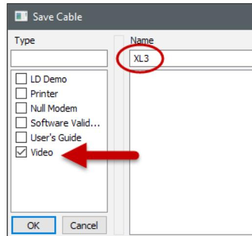
When saving multi-headed cables or wire harnesses, the *Connector Name* you apply to each connector may be helpful. We assign the default names J1, J2, J3, etc. to connectors in the order they are detected. If a custom pin map was active when you measured the cable, we use the names assigned in the map. Before saving, you may overwrite the default names by entering any changes on the right side of the *Save Cable* dialog under "Save Name", as it appears below.
