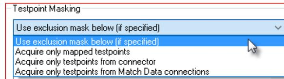
The Testpoint Exclusion Lists is a list particular testpoints that the CableEye software should ignore when interpreting raw data received from the tester. You can specify the default list to use in this field.
