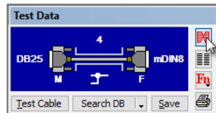
3. To examine the wiring of the cable in detail, **click the View Wiring** button. You will see the complete schematic of the cable along with connector and pin information. Use the ↑ and ↓ cursor keys to highlight a specific wire in the cable as shown below. This is helpful when reviewing the wiring of complex cables.
