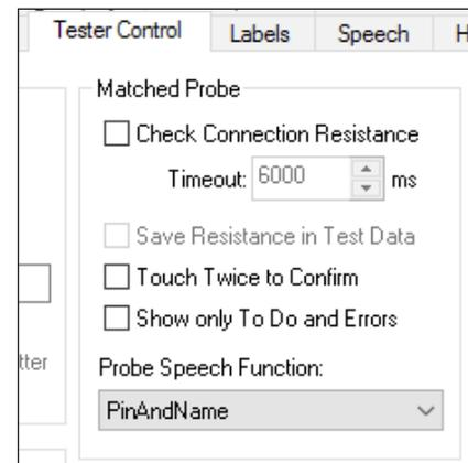
**Resistance Checked** - To enable this mode, **check** the **Check Connection Resistance** box.
