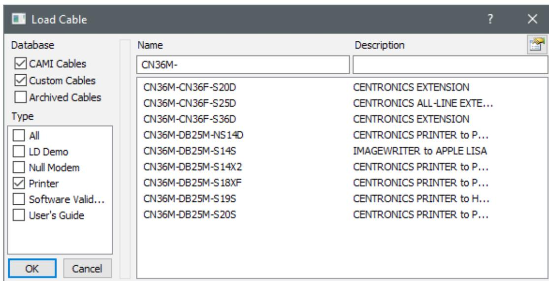
Any cables you load that have an embedded pin map name will *activate that map automatically* when loaded. In this case, you will see the Map file's name in red letters on the main screen. On the right, you see the map "BCP" has been activated with the cable file "Cable1".
