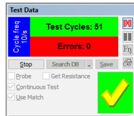
4. Flex the cable and connectors to locate intermittent connections. If any are found, a tone will sound, the error count will increment, and you will see a display with the intermittent connections highlighted (see below). In this case, we see an intermittent short between pin 15 and the shield.
