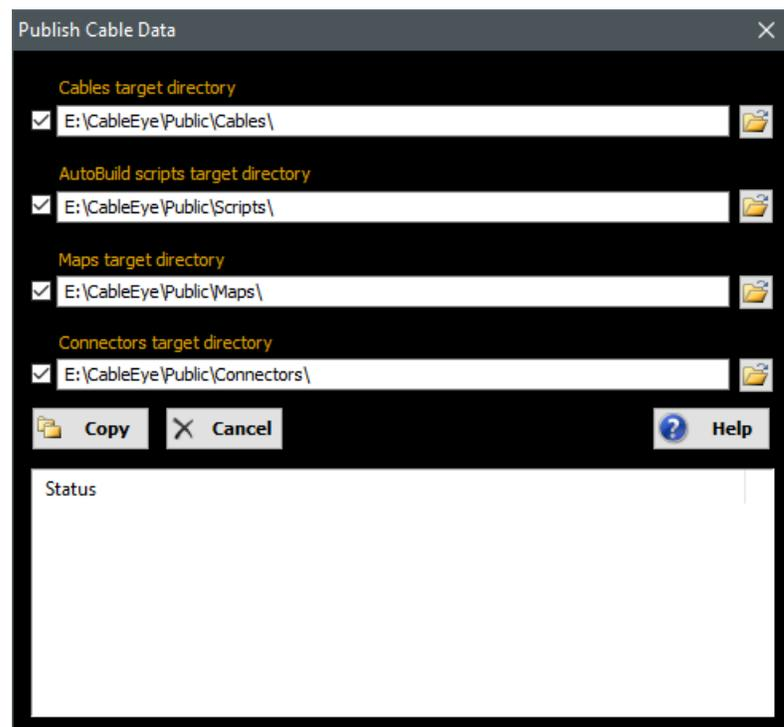
Click the Copy button to copy the cable files and any associated maps, scripts, or connector files to the specified shared locations.
