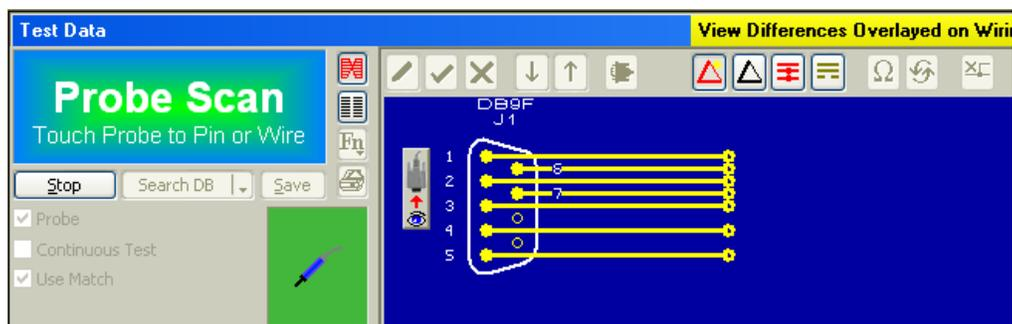
4. **Touch Pin 1** with the probe. This confirms the connection to that pin and the wire changes from yellow to white, and the system reads “One, Black”. Because the wire leading to Pin 1 should be black, the balloon appears with a black background which you may match to the wire between your fingers to check the color code.
