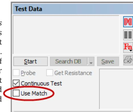
With *Use Match* checked, we use previously loaded or learned *Match Data* as a baseline rather than the first measurement of the test cable. Here, we DO test against a known standard, so if the cables are wired differently, *Continuous Test* will *always* fail regardless of whether the cable has intermittent connections.
