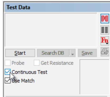
2. With the test cable attached, **click Learn Cable** to acquire Match Data. Once Match Data has been loaded, **click Start** to begin testing.
