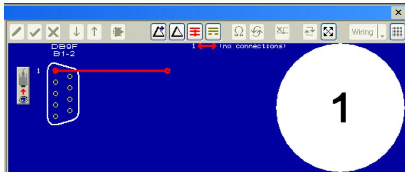
5. Continue probing and **touch all pins one at a time.** The last pin touched appears highlighted in red with all previously touched wiring remaining visible.
