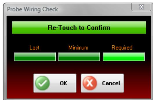
**Re-Probed Resistance Checked** - This is a combination of the previous two modes. The probed resistance must dip below the value as described in the *Resistance Checked mode*. An initial success tone is then played. The operator must then remove the probe from the lead and re-probe it in order to confirm the wire as Good.
