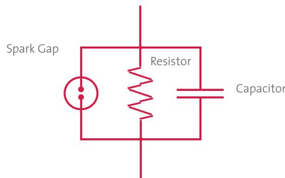
Figure 1: Basic insulation scheme in electrical products
