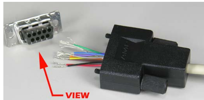
View of a DB9 Female connector looking INTO THE TERMINATIONS
