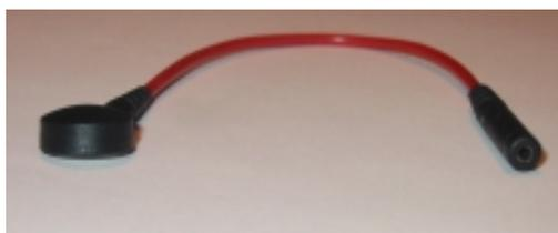
**SINGLE PIN TO SNAP WIRE CONVERTER**
