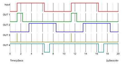
OUT 1 and OUT 4 demonstrate the use of the digital capacitor and resistor to create a single pulse. OUT 2 is the output of a delay circuit.
