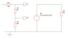
In the above circuit the voltage across B1 will be equal to the product of the voltages at nodes n1 and n2.
