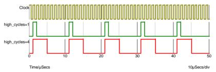
The above was carried out with I\_COUNT=0. I\_COUNT is the initial value of the internal counter. The output first goes high when it attains a value of 1 or 1+DIVIDE\_RATIO so when I\_COUNT is zero (the default) the output first goes high after the first rising edge. If I\_COUNT is set to 5 the output first goes high after the 6th rising edge and if I\_COUNT is -20, the 21st rising edge.
