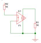
In the above circuit, the current in the output of F1 (flowing from top to bottom) will be 0.1 times the current in R2.
