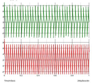
The top trace is without threshold control and the bottom trace is with it.
