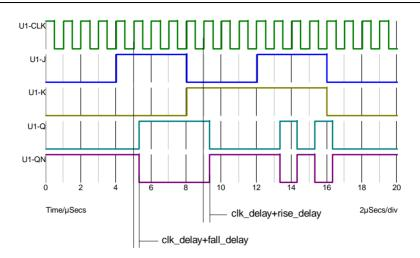
The following table describes the operation of the device when both inputs are at known states: The output can only change on a positive edge of the clock.
