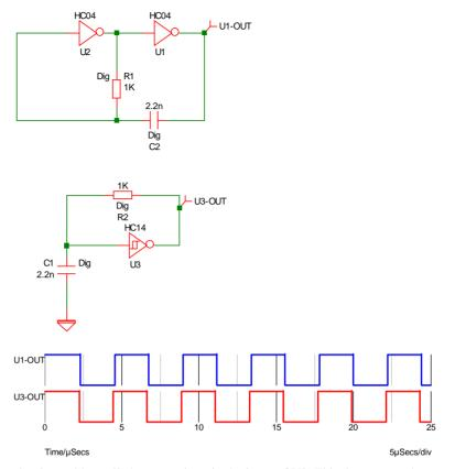
The first circuit would usually have a resistor in the input of U2. This does not work when using the digital R's and C's.
