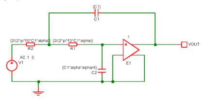
The above circuit is that of a two pole low-pass filter. C1 is fixed and R1=R2. The design equations are:
