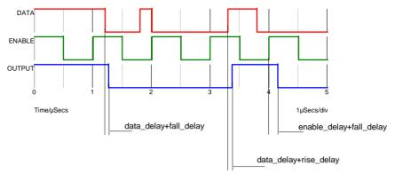
The asynchronous inputs (set and reset) override the action of the enable and data lines.
