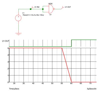
The graph shows the input and output of the NAND gate. Because the input is analog an implicit AD interface bridge will have been connected by the simulator. In the above example the parameters for this bridge have been set to:
