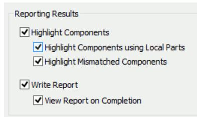
The **Highlight** options use the three colours on the Highlights page of the Colours dialog to indicate Pass, Warning and Fail status on the components that are checked.
