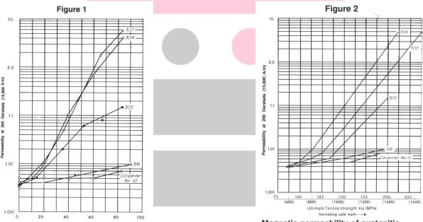
When cold working is employed, some normally nonmagnetic austenitic steels become substantially ferromagnetic
