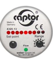
Measuring range adjusted to 3 m/s = 100% (9. LED)
