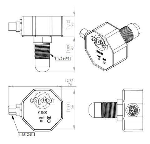
Figure 1. Dimensional Drawings (30mm NPT shown)
