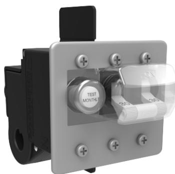
1-3 poles, up to 30 amps @ 120VAC & 120/240VAC max current & voltage, up to 5,000 amps max interrupting capacity.
