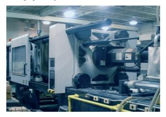
Generally, safety gates need a safety system guaranteeing top reliability and durability. In plastic machines, the main gate must be often opened – i.e. when the moulded part is not correctly released or at the end of each use – and safety must not be a problem. NES02 and NES13 simply solve the problem allowing the opening of the press motor mains, when the gates are open.
