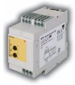
Measuring the regenerated voltage on a motor's coils, is the best way to determine if the tool on a motor's shaft is moving. This operation must be performed safely in order to comply with safety category 3. The MF1C provides this function, allowing for the opening of the lock of a safety gate only when the motion of a motor has come to a complete stop.
