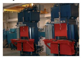
Presses are dangerous machines, because no gate can be used and light curtains may not be practical. The only way to guarantee safety is to make sure the operator has both hands busy when the machine is in operation. Safety category III C, complying with EN 574, allows ND12D to be used in the most demanding applications.
