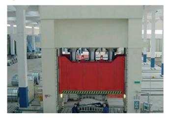
Safety light curtains are widely used in order to protect the working area of presses and punching machines. The Master- Slave cascade connection of the SB4M-SB4N Series provides protection in the dangerous areas and detects presence of operator. All the electronics for Slave unit monitoring (SB4N) are included into the Master (SB4M). Thanks to Carlo Gavazzi's solutions, mounting, wiring and set-up are quick and safe.
