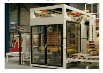
The safeguarding of packaging applications often requires that objects such as feed stock, work pieces etc. pass through the sensing field, without the activation of any stop signal. Carlo Gavazzi's SB4B Series light curtains allow up to three adjacent beams to be interrupted at any location along the sensing field. This system operates without triggering any safety output, such as floating or blanking. Quick and safe setting is ensured, thanks to the integrated DIP-switches.
