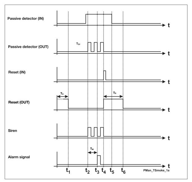
The above illustration shows the normal sequence and reset of an alarm:
