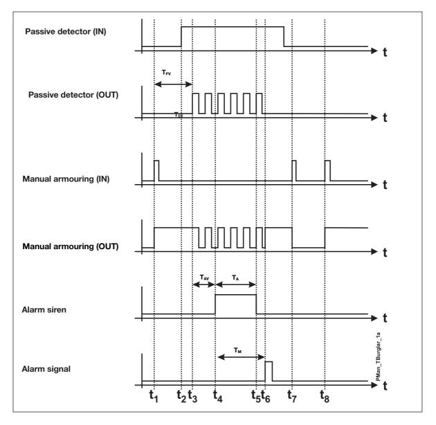
The above illustration shows the normal sequence of an alarm as well as early acknowledgement and the switching of the system back into the alert state through the Manual Armouring option:
