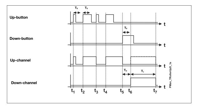
The above illustration is based on a roller blind application with adjustment of tilting blinds (Reverse Up time  $T_v$  of 3 s).
