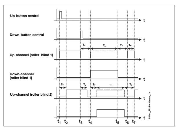
The above illustration is based on a roller blind master application with sequential operation mode and a Reverse Up time  $T_{R}$ .
