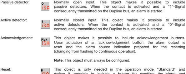
This object is only needed in the operation mode "Standard" and makes it possible to include a button for resetting the alarm and restarting the system. This requires prior acknowledgement of the alarm.
