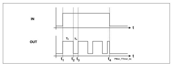
The impulse is generated shortly after the input has switched on at time  $t_1$ . A pulse cycle consists of the Ontime  $t_E$  and the Off-time  $t_A$ . When the input is switched off, the pulse cycle also ends.
