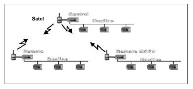
The Radio Modem must be connected to the COM2 of the Master Generator. For serial cable pin connections, please refer to the Master Generator datasheet. The baud rate selected for COM2 must correspond to the baudrate used by the radio modems and the other master generators in the network.
