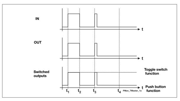
The master function remains active until the input is switched off. In the above example, the outputs switch on, and - in the case of a push button function - remain on, until the master function switches off again.
