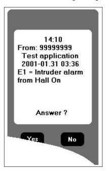
If more dial-out phone numbers have been defined, an acknowledgement can be sent to the Generator by sending an empty SMS message back. The Generator will then stop sending messages to the following phone numbers.
