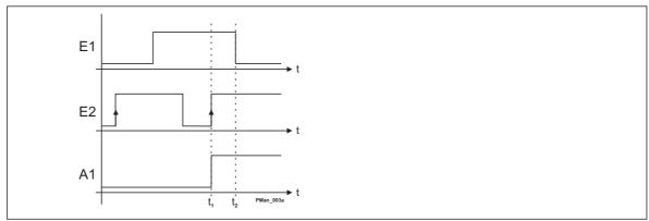
Output A is only active, when input E1 is active and input E2 is not active (range between the dotted lines). The internal processing in the Master Generator inverts the value of E2 before it is output (ie sees it as active).
