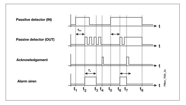
The above illustration shows the normal sequence and reset of an alarm in the operation mode "Auto reset":
