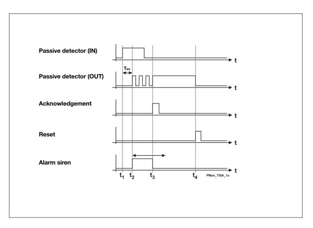
The above illustration shows the normal sequence and reset of an alarm in the operation mode "Standard":
