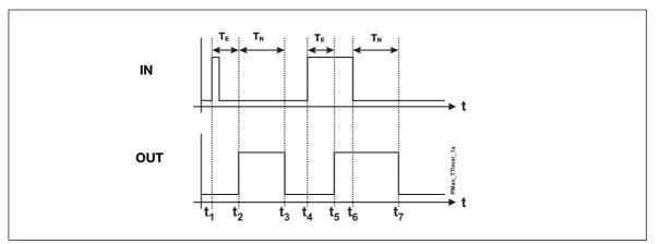
The on-delay  $t_E$  starts shortly after the input signal at time  $t_1$ . After elapse of the delay, the On-time  $t_N$  starts. After elapse of the On-time ( $t_3$ ), the output switches off again. To achieve this, the input must be reset before time  $t_3$ .
