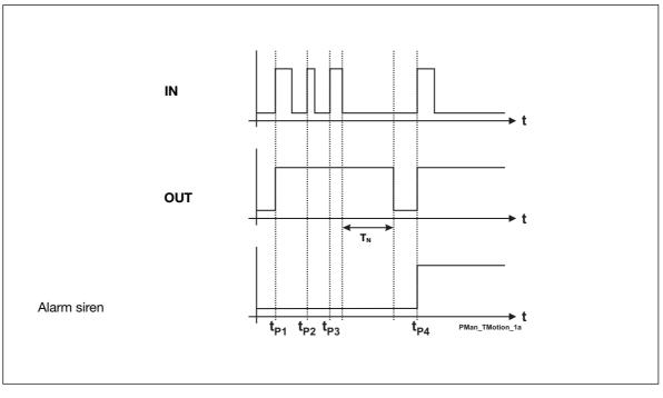
$t_{P1}$ ,  $t_{P2}$ ,  $t_{P3}$  and  $t_{P4}$  are the points of time at which the motion detector generates a signal. The impulse duration depends on the characteristics of the detector.  $T_N$  is the set off time retriggered by the impulses  $t_{P2}$  and  $t_{P3}$  and therefore only begins after elapse of the third impulse.
