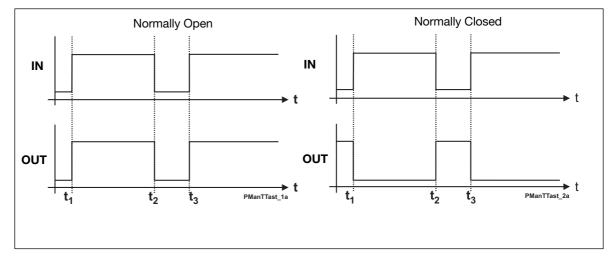
The output follows the input upon a short delay. In the Normally closed function, the output function is the opposite of the input function.
