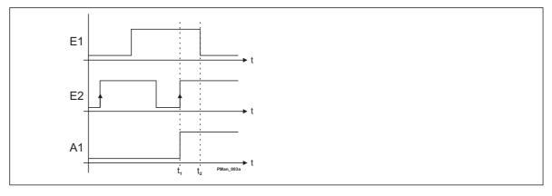
Two conditions must be fulfilled (AND): E1 must be active and E2 must trigger on leading edge. This only takes place at t1 (the dotted line to the left). If the signal on E1 goes Off (dotted line to the right), output A will also be reset.
