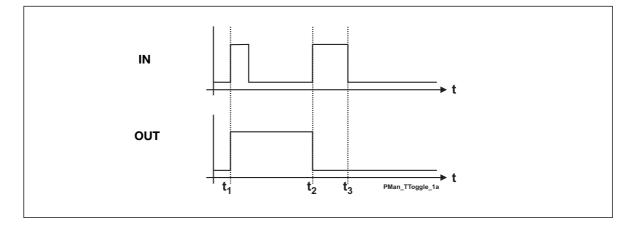
The first triggering of the input switches the output on, the second triggering switches the output off again.
