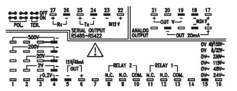
Connect MDI40A (ammeter) as shown in the figure. <u>Attention: the</u> <u>ammeter input is to be connected in series to the source to be measured</u>.
