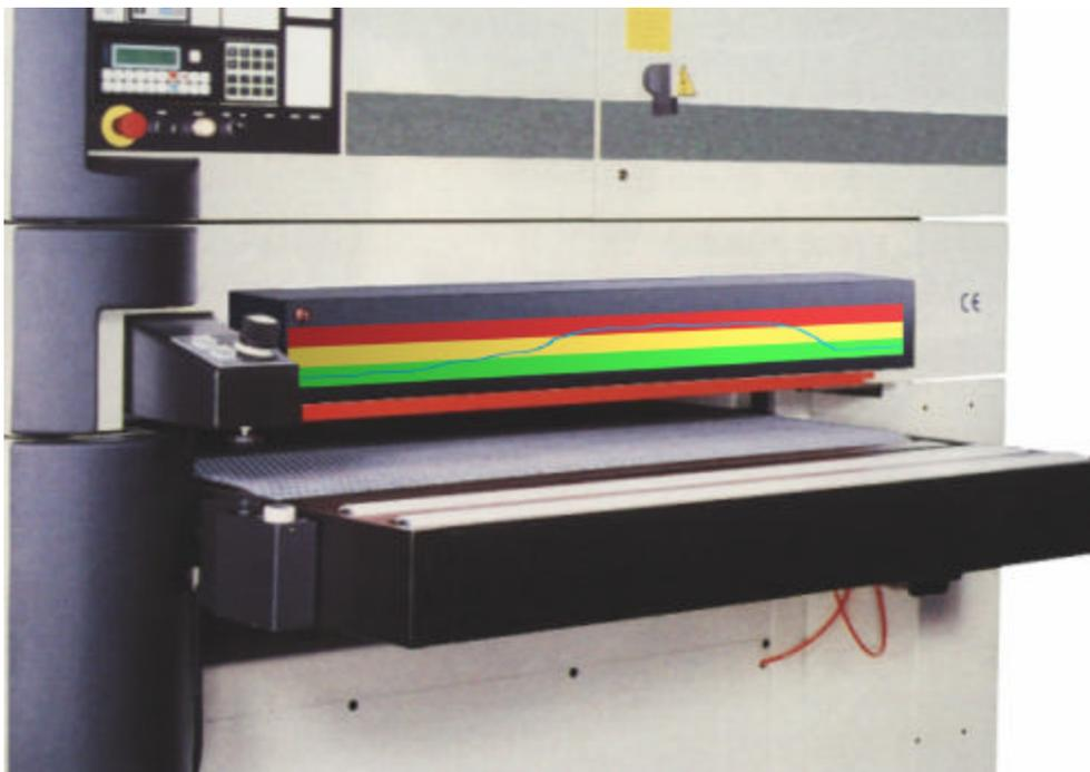
The new SandTrac belt monitoring device prompts operators to even out utilization of abrasive belts with an easy-to-use graph and scale.
