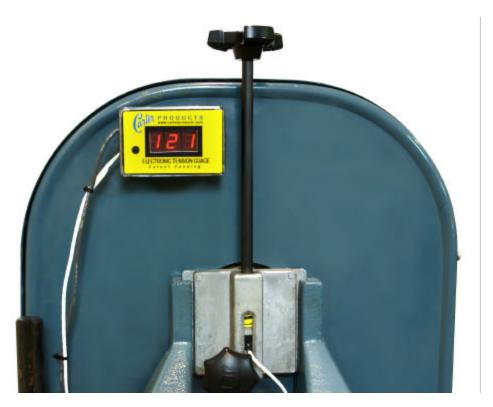
The new ETG<sup>™</sup> shows the user the exact tension of their band saw blade at all times with an easy-to-use digital read-out.
