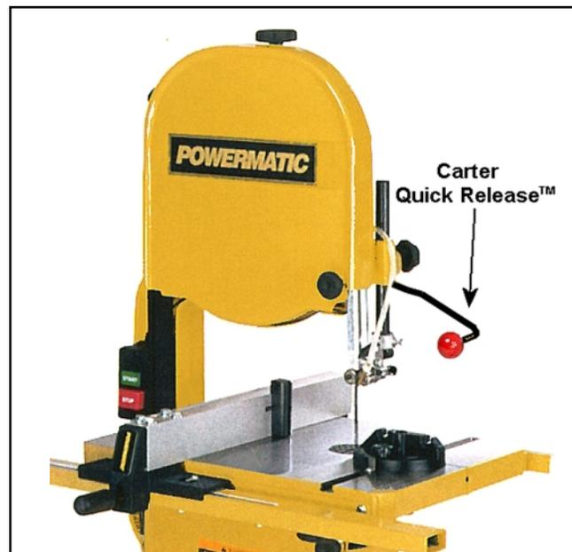
The Carter Quick Release Bandsaw Blade Tension Toggle will be standard equipment on the new PowerMatic 14CS saws. The Quick Release extends blade and saw life and improves safety.
