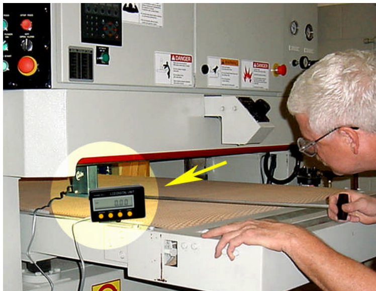
The Carter Widebelt Sander Set-up & Diagnostic Device makes precise calibration of the sanding platen quick and easy.
