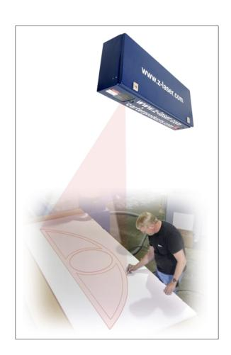
Get a free video of the Carter CPS Precision Laser System. Here the CPS outlines the path of the cutting tool on a CNC router. The CPS is a powerful productivity tool for any operation where critical positioning is required.
