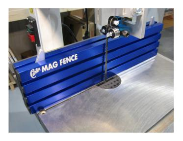
The new Carter MagFence<sup>TM</sup> is a fast, easy, cost-effective alternative to other bandsaw rip fences on the market today. Powerful magnets hold it in place, it is infinitely adjustable, and requires no hardware or saw modification.
