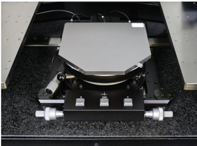
Figure 19. The chuck stage available on the EPS200RF is designed with integrated coarse X/Y movement, fine X/Y positioning and fine-theta adjustment
