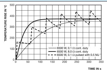
Standard GRE1Jxxxxx 6500 W grid banks are rated with max. design temperature rise of 375 °C over an ambient.
