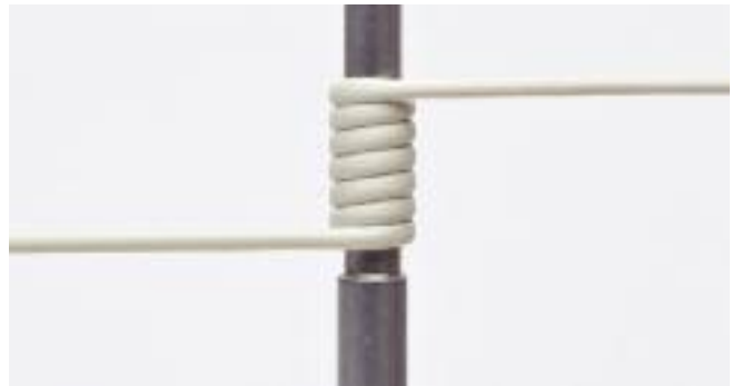
Figure 4.4a – ClearCurve Rugged Drop Cable Wrapped Around Mandrel | Photo CCV010
