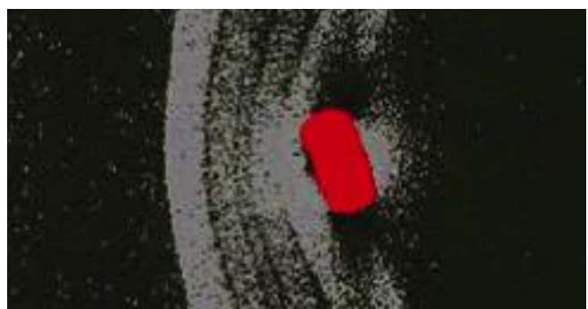
Figure 4.4c – X-Ray of Stapled ClearCurve Rugged Drop Cable | Photo NS156
