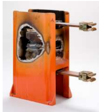
Figure 5. Failed vacuum interrupter
