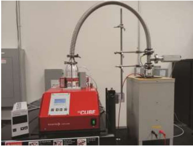
Figure 10. Test setup for developing vacuum versus current data
