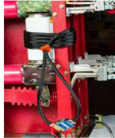
Figure 8. A newly-designed flexible, magnetic coil for field testing
