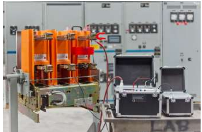
Figure 9. Rigid, magnetic coil applied to an entire pole
