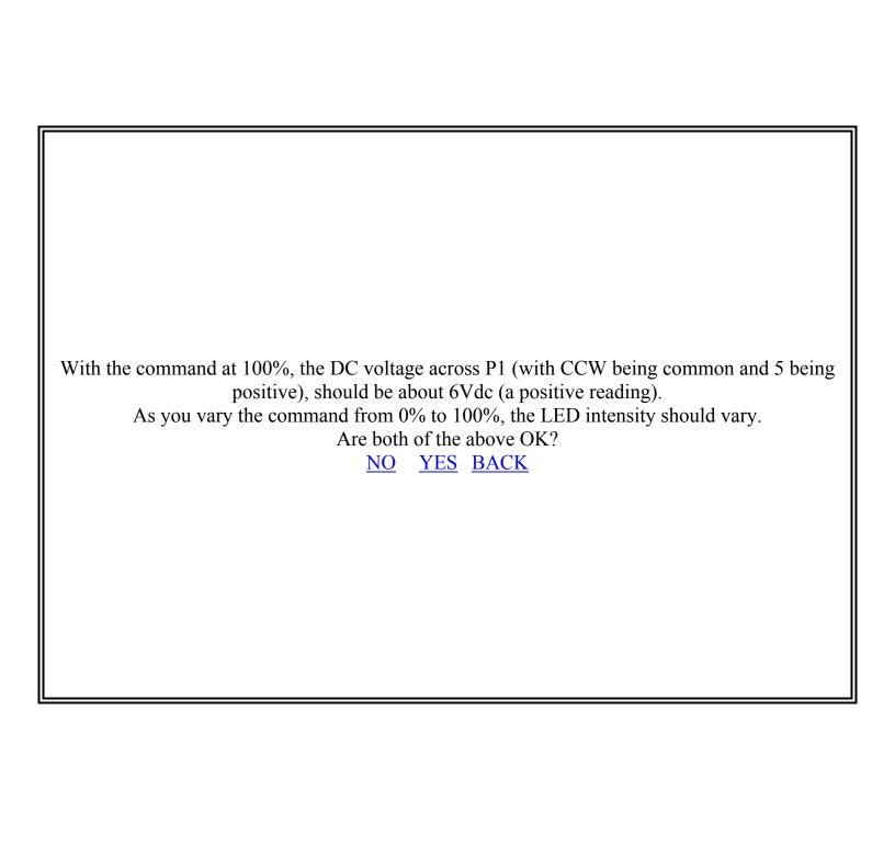
With the command at 100%, measure the DC voltage across P1 as follows: Use CCW as common for all readings in this step.
