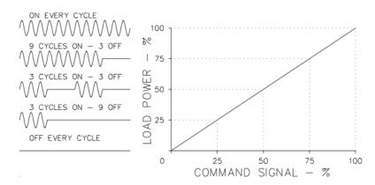
to obtain the desired load power with infinite resolution. At 50% power the 3021A controller is ON for 3 electrical cycles and OFF for 3 electrical cycles. At lower power levels load power is applied for 3 cycles and the number of OFF cycles is increased.
