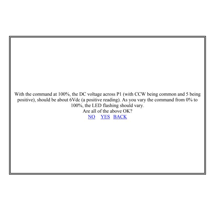
With the command at 100%, measure the DC voltage across P1 as follows: Use CCW as common for all readings in this step.
