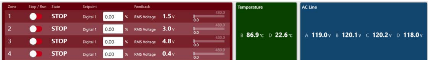
Figure 4.10: Condensed multi-zone dashboard for a FUSION controller.
