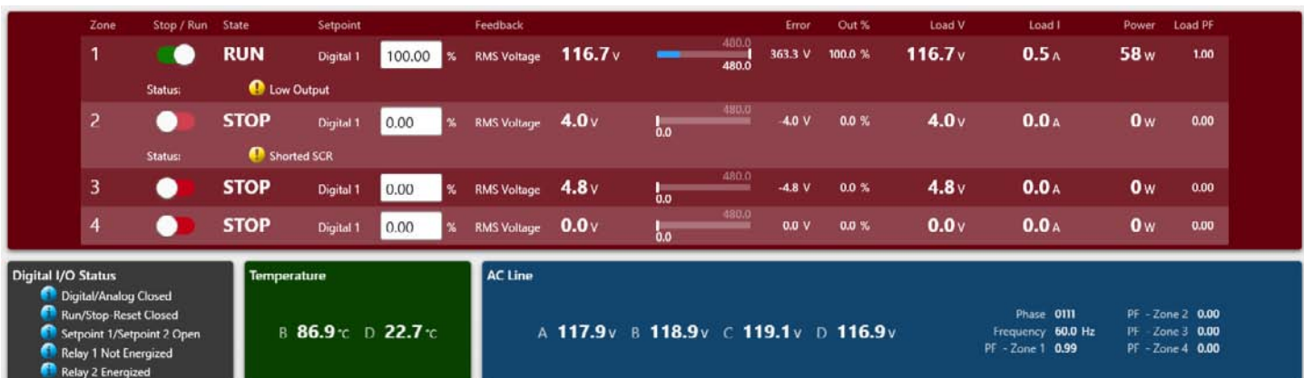
Figure 4.11: Detailed multi-zone dashboard for a FUSION controller.
