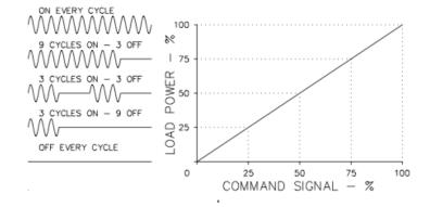
to obtain the desired load power with infinite resolution. At 50% power the 3021A controller is ON for 3 electrical cycles and OFF for 3 electrical cycles. At lower power levels load power is applied for 3 cycles and the number of OFF cycles is increased.
