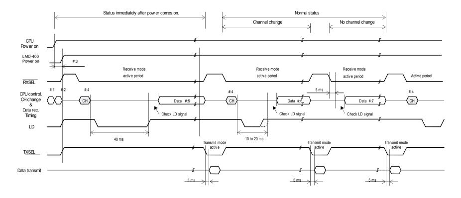
Figure 3: Timing diagram for LMD-400
