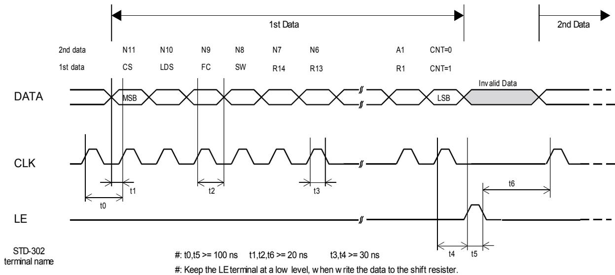
The PLL IC, which operates as shown in the block diagram in the manual, shifts the data to the 19-bit shift register and then transfers it to the respective latch (counter, register) by judging the CNT control bit value input at the end.
