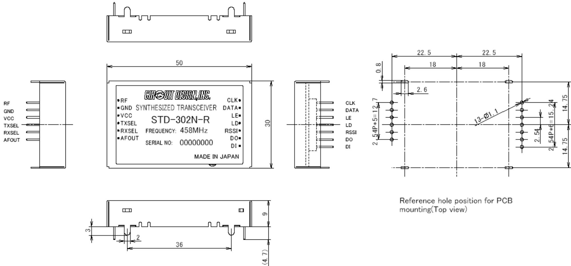
Reference hole position for PCB mounting(Top view)
