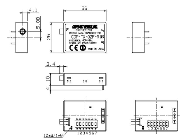
Reference hole position for PCB mounting (Top view)
