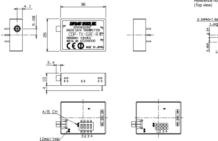
Reference hole position for PCB mounting (Top view)
