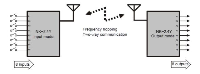
The NK-2.4Y operates with low voltage and low current consumption, achieving long time operation on two 1.5V AA batteries. Operation on one lithium coin battery (CR2032) is also possible.
