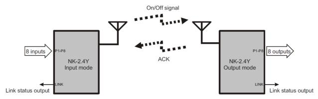
It is also possible that the Output-mode module continuously outputs signal as long as the button switch connected to the Input-mode module is pressed.
