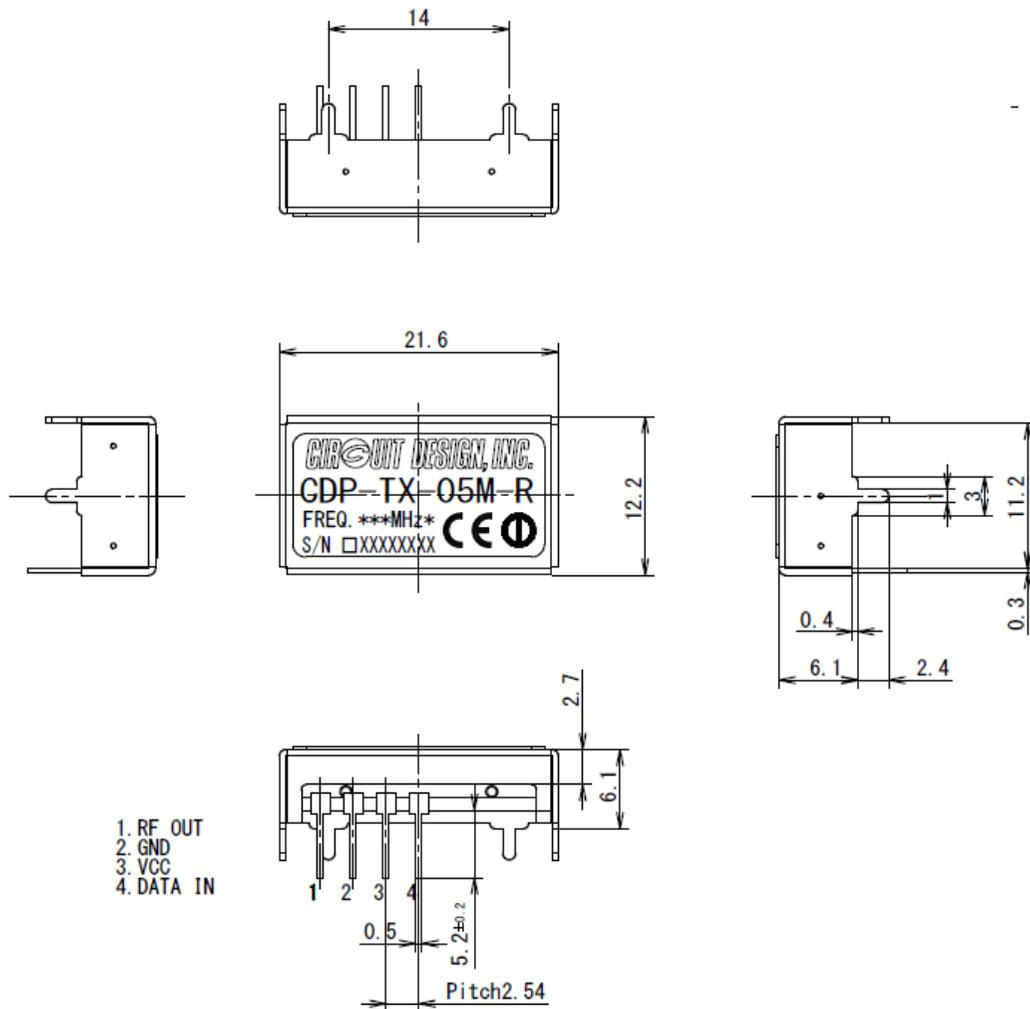
Reference hole position for PCB mounting
