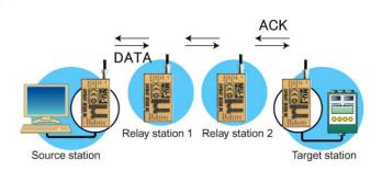
The MU-1 is a serial data communications modem designed to offer the reliability, shock resistance, vibration resistance and high quality required for use in industrial applications. The MU-1 uses the UART serial interface to interface with the host system, while data input/output is performed with simple commands.
