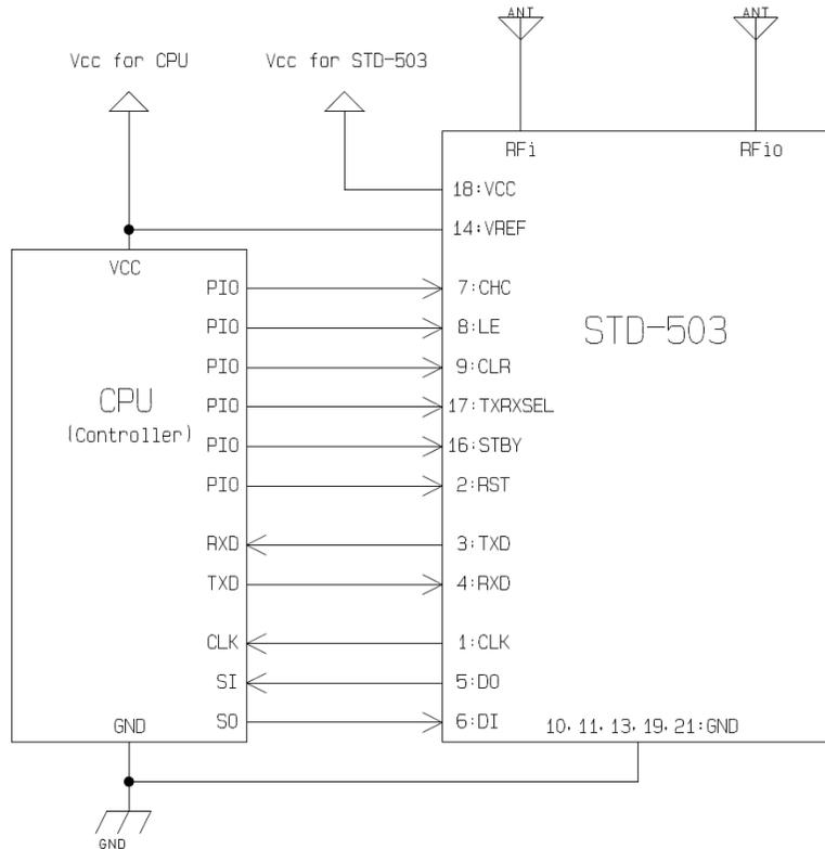
Using a different VCC voltage for the CPU and the STD-503
