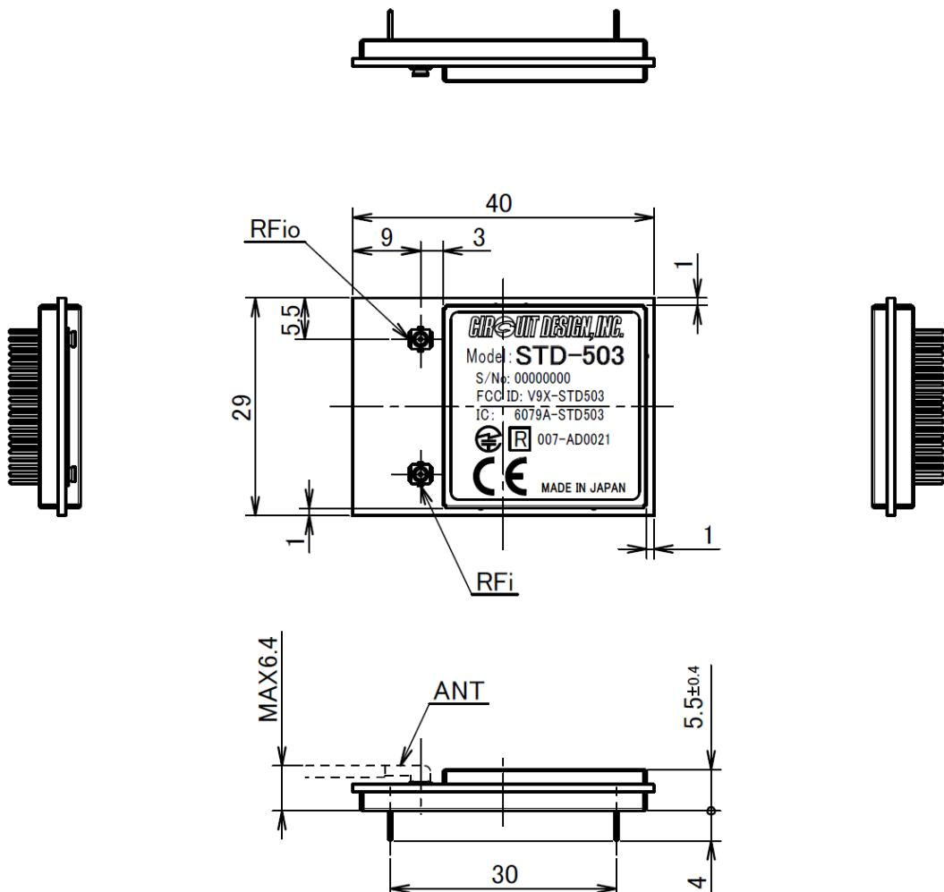
Reference hole position for PCB mounting
