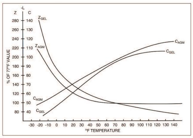
Figure 6-Impedance and Conductance VS. Temperature
