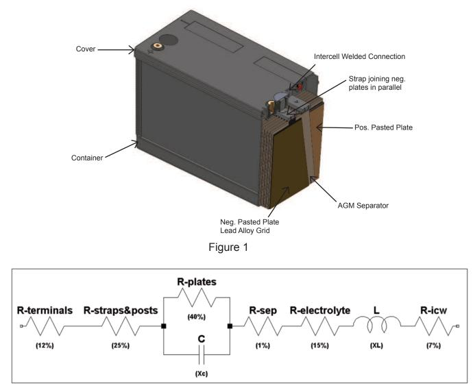
FIGURE 2 - Battery Equivalent Circuit
