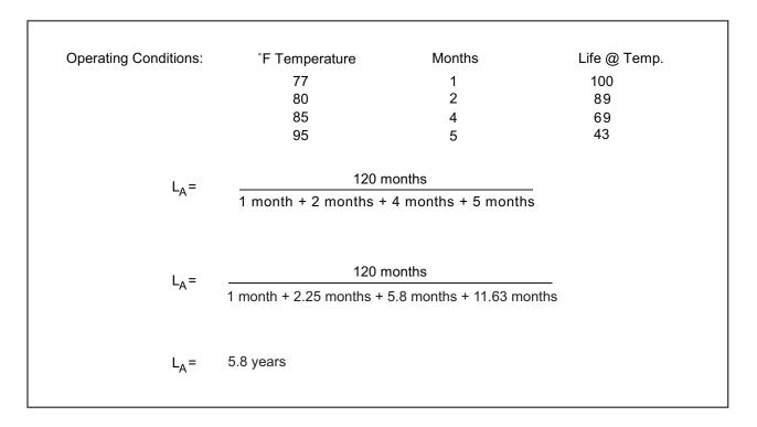
As can be seen, the affect of elevated temperature upon the life of the battery is dramatic and the desirability of a temperature compensated charger and/or cooler environment is evident.
