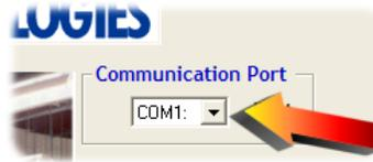
Each computer may have differing numbers of communications ports available. Some communications ports will be shown that use a modem, others will use the 9-pin serial port on the back of the computer.
