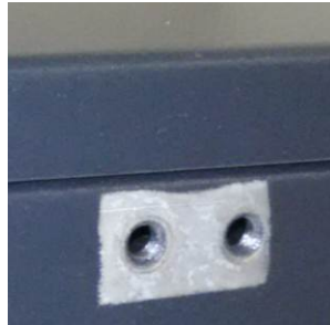
Case ground connection on rear of battery
