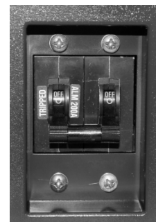
Circuit Breaker on front of battery
