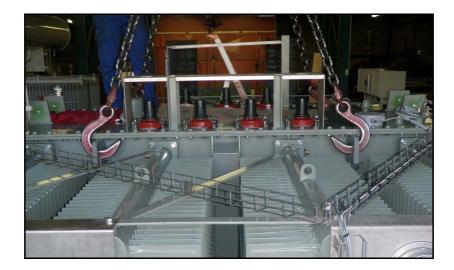
When unloading, the rollers must be mounted on the substructures and tilted in the desired direction. The yokes are stopped from turning using the envisaged screws. The unit must be laid down delicately on the floor.
