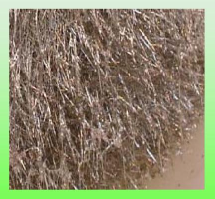
Photo's showing copper dendrite formation during R&D copper skimming trials
