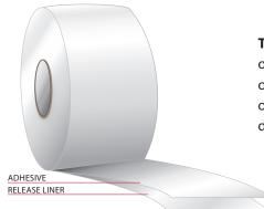
**Transfer tapes** or unsupported tapes have a coating of adhesive on one side of a double sided release liner. There is no additional backing or supporting material. These tapes can be converted into other types of tape product by lamination to another material, or can be used directly to bond two materials together.
