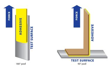
tape is applied to the surface with a defined amount of pressure and then allowed to remain on the surface for a controlled amount of time (often 20 minutes but tests using 24 hours, or more are also performed).
