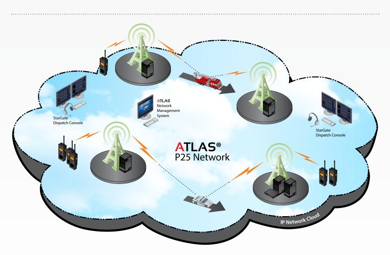
**EFJohnson's** ATLAS P25 infrastructure solution utilizes a unique, flexible, distributed, and scalable IP based architecture designed to meet mission critical needs. ATLAS system solutions are flexible and designed to fit the specific needs of each customer whether it is a greenfield system deployment, migration from proprietary technologies, or evolution from analog to a digital P25 system.
