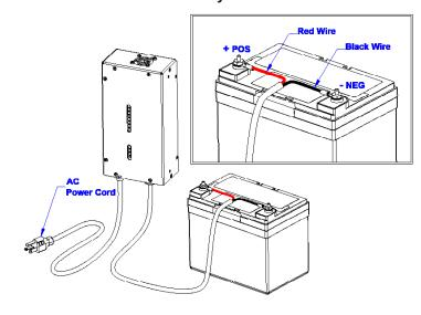
□ When connecting two batteries in series, it is imperative that the amount of charge and discharge be equal for both batteries. If there is an imbalance during charge or discharge, excessive battery voltage will occur. This results in an overvoltaged battery and causes dangerous battery out gassing and destruction. For accurate charge balancing, use a dual bank charger, such as CT500 or TPRO series.
