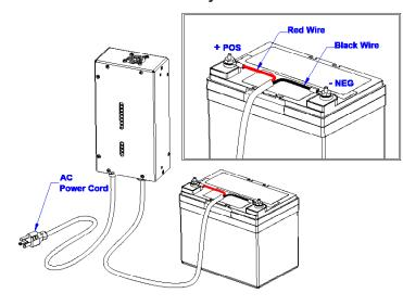
□ When connecting two batteries in a series, it is imperative that the amount of charge and discharge be equal for both batteries. If there is an imbalance during charge or discharge, excessive battery voltage will occur. This will result in an overvoltaged battery and will cause dangerous battery out gassing and destruction. For accurate charge balancing, use one of our dual output chargers, such as the CT500 or TPRO series.
