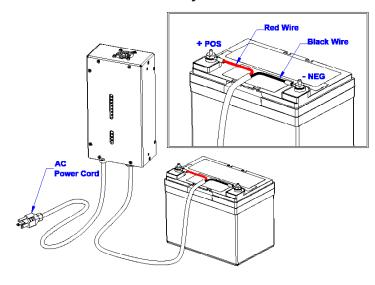
□ When connecting two batteries in series, it is imperative that the amount of charge and discharge be equal for both batteries. If there is an imbalance during charge or discharge, excessive battery voltage will occur. This results in an overvoltaged battery and causes dangerous battery out gassing and destruction. For accurate charge balancing, use a dual bank charger, such as CT500 or TPRO series.
